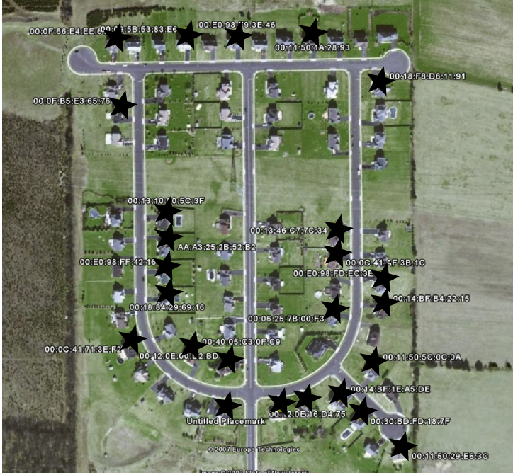
Fig. 5. Orthophoto-based geocoding for the postal addresses along with the MAC address of the AP installed in that address
